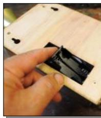
**2** Ease the battery holder top first from the enclosure and insert 4 x AA batteries. Don't clip it back into the enclosure yet, as the horn will sound if the copper cable wires touch together! Clip it back into the enclosure once installation is complete.
