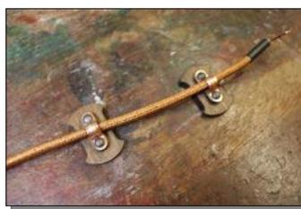
**4** Thread the copper coloured cable through the cable supports.
